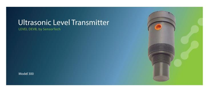
The model 300 is a four wire, 24 VDC 4-20ma level transmitter based on the concept of ultrasonic pulse operating at 52 KHz/70KHz and mounts on top of tank looking downward. The time of flight is measured many times to construct an average of the true distance measured.
