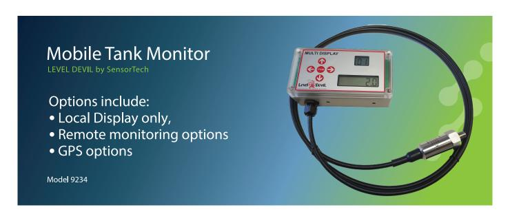
The model 9234 liquid level gauge is a battery-powered local display and controller that mounts on a single tank, or near it – measuring liquid levels with a hydrostatic pressure sensor. The pressure sensor, on the end of the cable, may enter the tank from the top (submerged in the liquid), or may be connected to a port opening on the exterior of the tank, at its base.
