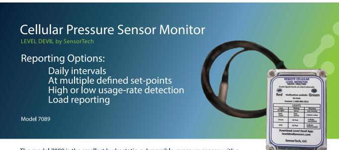
The model 7089 is the smallest hydrostatic, submersible, pressure sensor, with a cellular remote commu-nicator, on the market. Its five year battery, with an amp booster, required during cellular transmissions, makes it maintenance free and dependable. Field programmable scheduling and adjustable reporting is standard on this and all Level Devil® field devices. Different sensors and cable-materials are available to help serve a wide market of liquid level needs.
